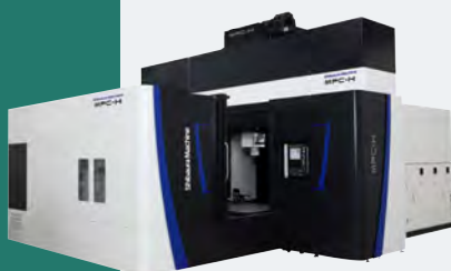
Double column type machining center (MPC-H)
