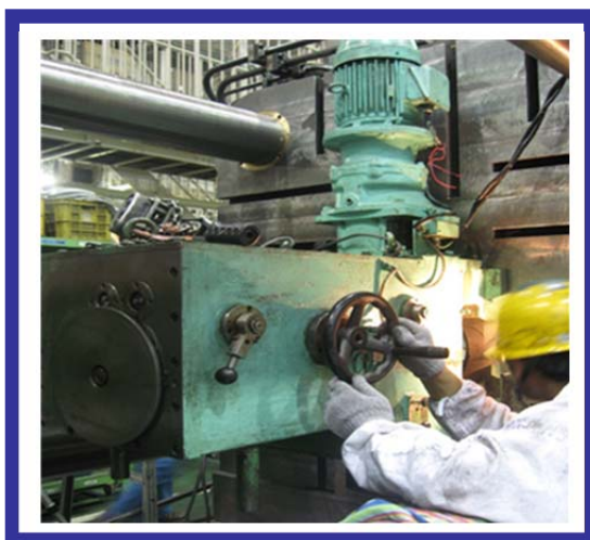
射出口加工 Injection Port Machining
